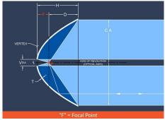
An electroformed parabolic reflector is a parabola-shaped reflective surface used to collect and direct wave energy such as light.
